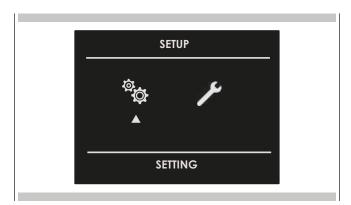
2. Use this menu to change the following settings: Press the keys  $\triangleleft \triangleright$  or  $\triangle \nabla$  to select the setting or change a sub menu from among the six available ones and confirm by means of the  $\boxdot$  key.
