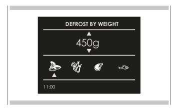
Select the type of meal using the arrows  $\triangleleft$  and  $\triangleright$ , then set the weight using the arrows  $\triangle$  and  $\nabla$ , finally start thawing using the key  $\boxdot$ .
