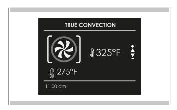
Just as soon as the set temperature is reached, an acoustic signal is heard and the instantaneous temperature indication disappears.
